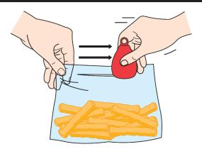
Gently squeeze jaws together and slide Viper away from your body to make a cut along the top of the material. To maximize effectiveness, replace Viper when reduction in cutting performance is identified.
