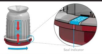
Align release button with ridges as shown. Rotate base past lock tab (listen for audible "click"). Tighten base until seal indicator is within the seal zone.
